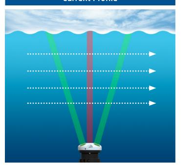
The AWAC uses the three slanted beams to measure the current profile over a range determined by the acoustic frequency. Large transducers transmit narrow acoustic beams and provide accurate data. The AWAC will alternate between wave data collection and current profiling. If the wave data collection is longer than the interval between current profiles, the AWAC will skip a current profile to ensure continuous wave data. Please contact Nortek if concurrent wave and current information is required.
